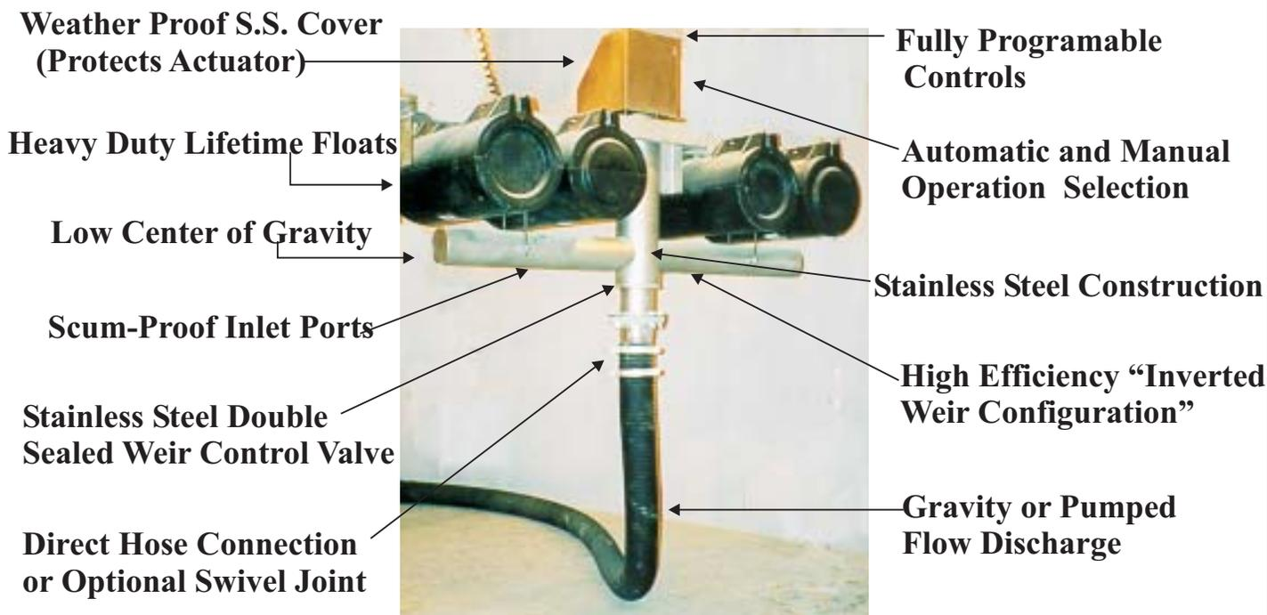
**AquaTec decaners are the only choice for SBR systems if low BOD and low effluent solids are required. No other decanter can offer the same efficiency. Their reliability in all weather & process conditions is unparalleled.**
